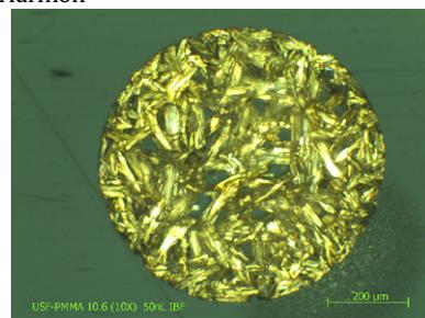
**Liquid–liquid phase separation in a polyethylene blend monitored by crystallization kinetics and crystal-decorated phase morphologies**
